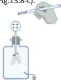
Fig.13.8 (a) Charging the electroscope positively
