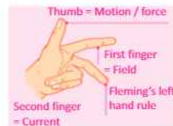
Fig. 15.7: Direction of force on a current-carrying conductor placed in a magnetic field
