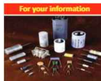
All of these devices are capacitors, which store electric charge and energy.
