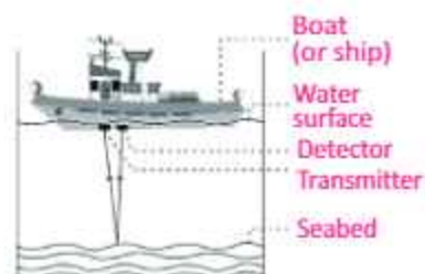
Fig. 11.14: Ultrasonics are used to measure the depth of water by echo method
