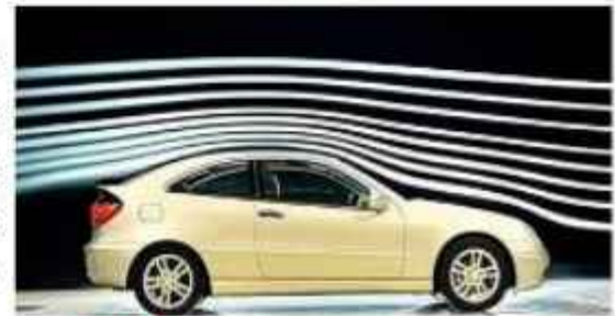
Fig. 3.25 Streamline air flow over a speedy car
